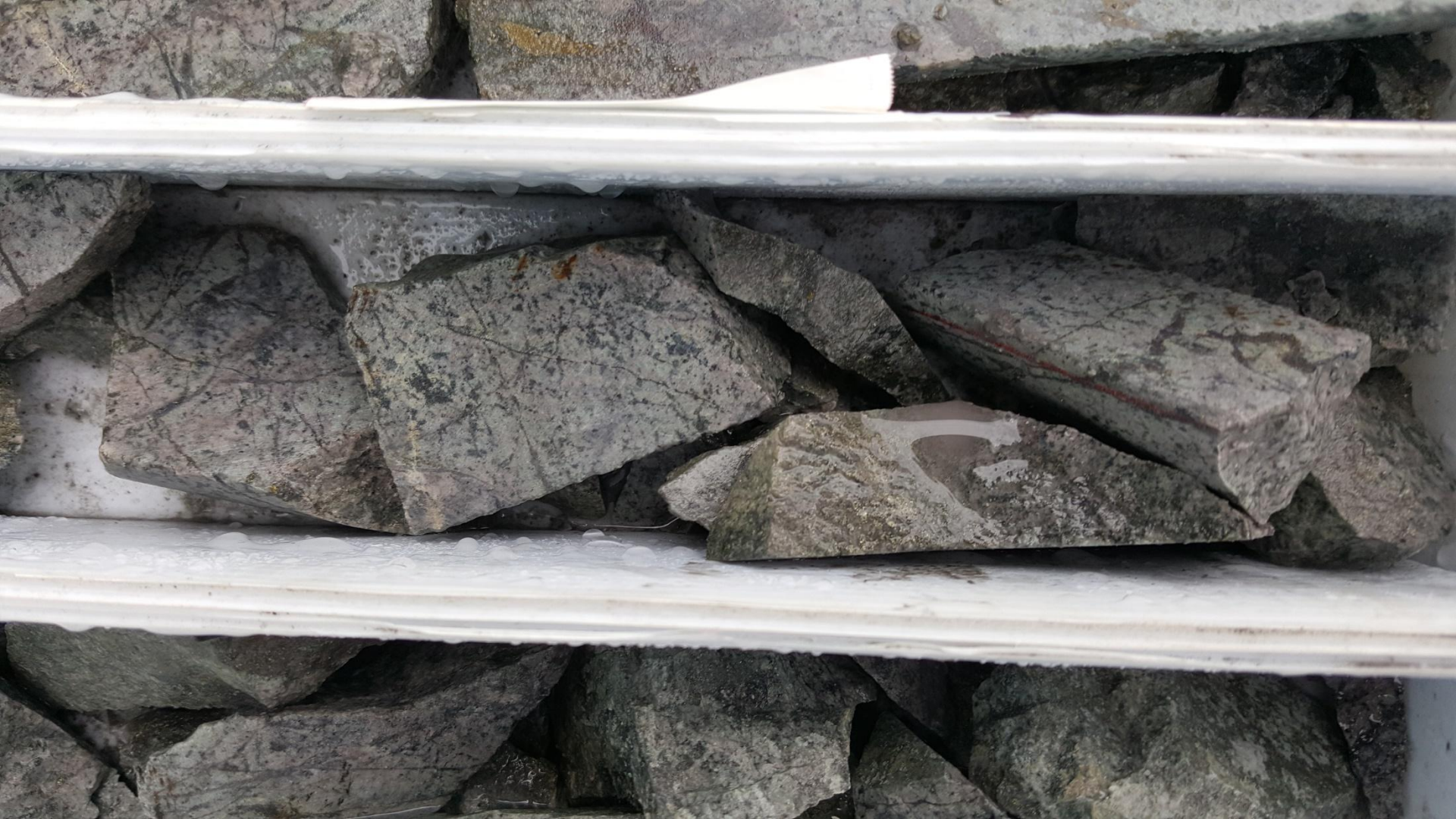
Hole EC-16-010 @ 293.0 meters depth Within a 1.5 m sample (292.0-293.5) that returned 0.51% copper and 1.89 g/t gold
